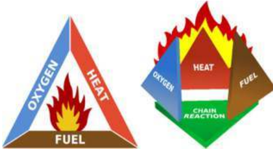
Figure 1 Fire Triangle and Fire Tetrahedron
