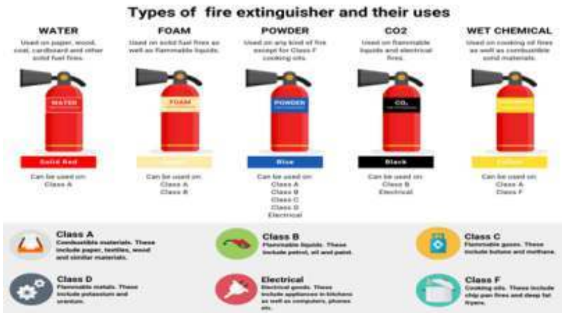
Figure 2 Types of Fire Extinguishers and Their Uses
